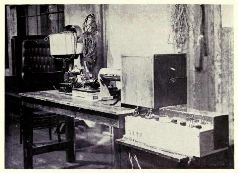
The first television camera set up in the Green Street laboratory
